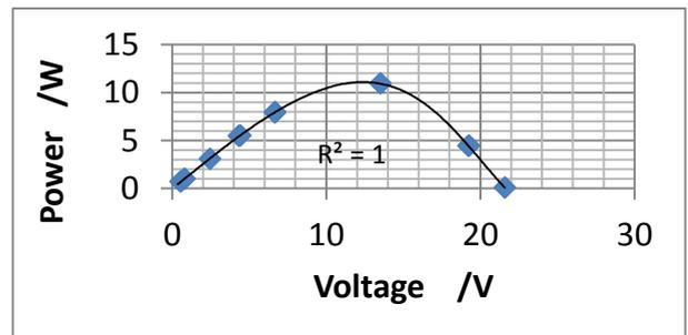
Figure 3: Power - voltage curve for module characteristics of figure 2
