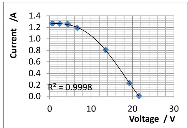
Figure 2: Current - voltage characteristics of the module at solar irradiance of  $813W/m^2$  and temperature of  $47^\circ C$ .
