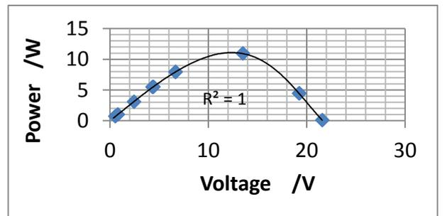
Figure 3: Power - voltage curve for module characteristics of figure 2
