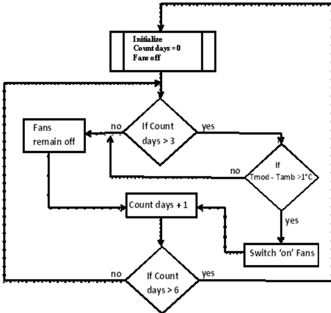
Figure 1. Flowchart for implementation of cooling of module. Note: Tmod and Tamb are module temperature and ambient temperature respectively.
