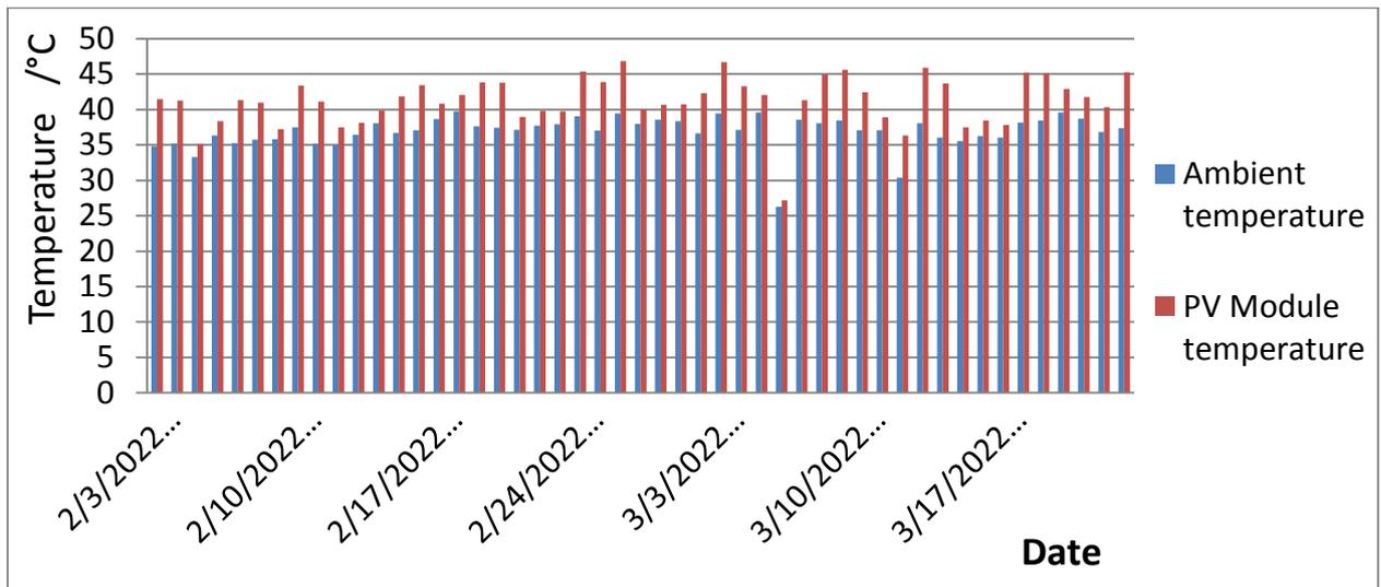
Figure 4: Profile of daily ambient and PV module temperatures.
