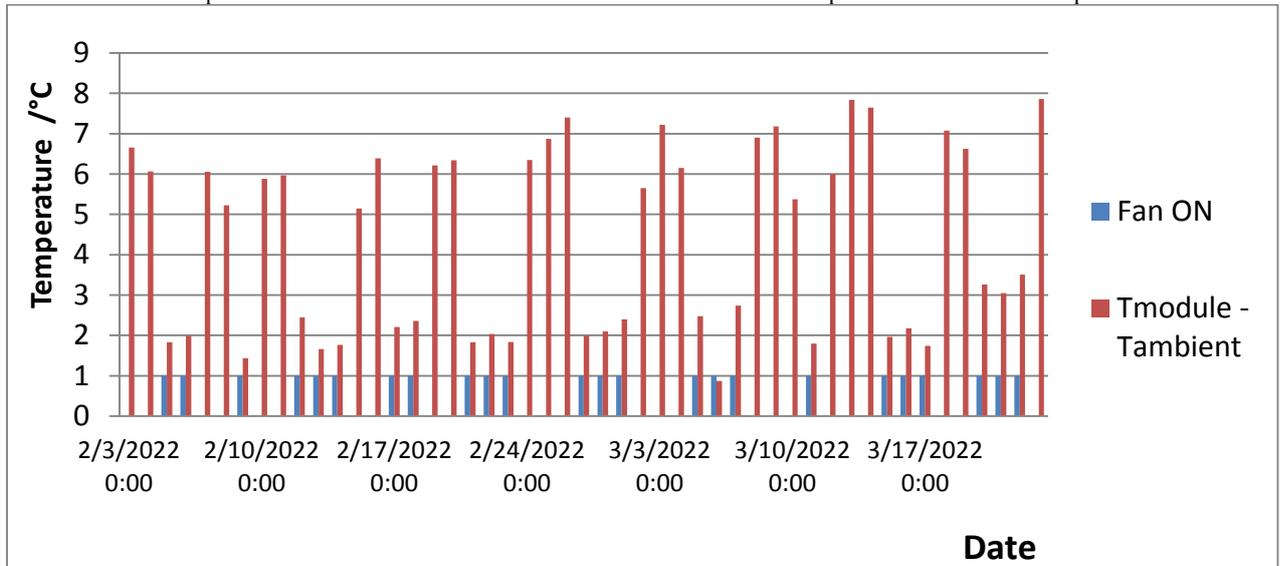
Figure 5: Profile of daily difference between PV module and ambient temperatures ( $T_{module} - T_{ambient}$ ) when fan is on and off. Days when fans are on present with lower values of  $T_{module} - T_{ambient}$
